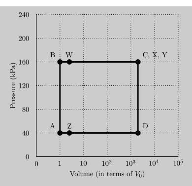
We start by computing pressures. The minimum pressure is attained when only the piston is to be lifted, so
