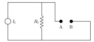
From the point of view of any passive resistance that is connected between A and B the circuits are identical. You don't need to prove this statement, but you do need to find  $I_t$  and  $R_t$  in terms of any or all of R and  $I_s$ .
