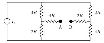
a. Connect an ideal voltmeter between A and B. Determine the voltage reading in terms of any or all of R and  $I_s$ .
