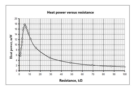
To determine the position of the maximum, it is necessary to take additional measurements in the range of 0 to 10 k $\Omega$ . According to the measurement results, it turns out that the maximum heat power generated in the resistor is reached at
