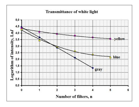
**3.2** It can be seen from the graph that formula (5) is correct for grey filters, but not for blue ones. The main reason for the violation of the obtained law is that the transmittance significantly depends on the wavelength of incident light. So, for grey filters, the transmittance varies little in the visible range of wavelength and formula (5) is applicable within the experimental error. For blue filters, though, the transmittance varies noticeably, such that formula (5) turns inapplicable.
