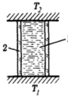
“1” is a water column, “2” is a heat insulating tube.
