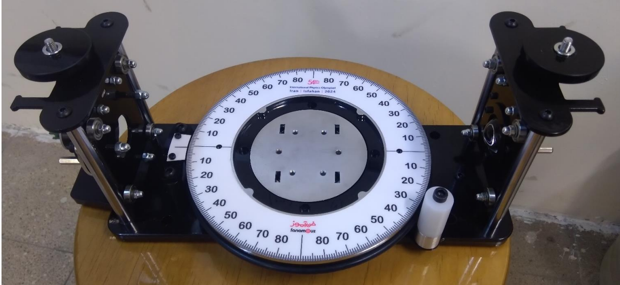
The main platform which consists of: Laser, Protractor, Magnifying lens
