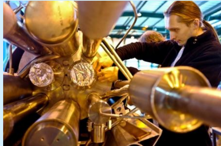
Installation of radiation detectors close to the magnets https://www.liverpool.ac.uk/opac/projects/cern/
