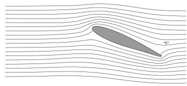
i. (0.8 pts) If the aircraft's ground speed is  $v_0 = 100 \text{ m/s}$ , what is the speed of the air,  $v_P$ , at the point P (marked in the fig.) with respect to the ground?
