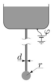
A long metallic pipe with internal diameter d is pointing directly downwards. Water is slowly dripping from a nozzle at its lower end, see fig. Water can be considered to be electrically conducting; its surface tension is  $\sigma$  and its density is  $\rho$ . A droplet of radius r hangs below the nozzle. The radius grows slowly in time until the droplet separates from the nozzle due to the free fall acceleration g. Always assume that  $d \ll r$ .
