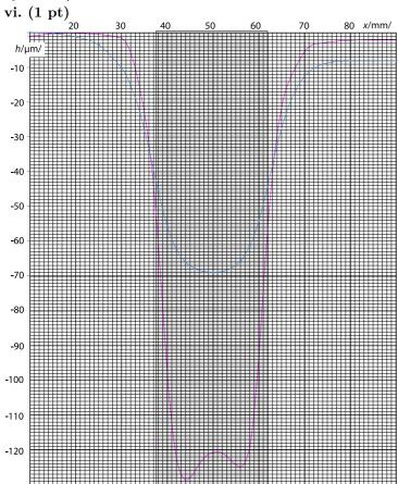
Similarly to the previous figure, blue curve corresponds to a water depth of ca 2 mm, (data given in the table above), and the violet one — to 1 mm.
