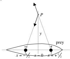
Assuming that the resistivities of the prey body and that of the surrounding seawater are the same, implying the elimination of the boundary surrounding the prey, the two spheres seem to be in infinite isotropic medium with the resistivity of  $\rho$ . When a small sphere produces current at a rate  $I_s$ , the current flux density at a distance r from the sphere's center is also
