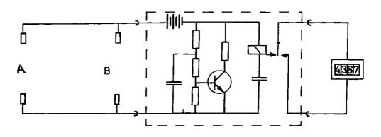
The purpose of the transistor circuit is to keep the relay position after closing of the contact at B, even if this contact is opened afterwards for a few milliseconds by a jump or chatter of the cylinder.
