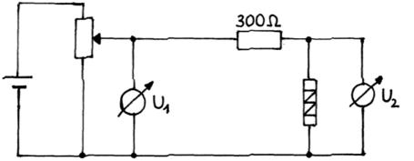
The graph of the function  $U_2 = f(U_1)$  has generally the same form for both directions of the current, but the absolute values are different. By requesting that the semiconductor element has to be placed in such a way, that the output voltage U<sub>2</sub> is as high as possible, a backward direction should be used.
