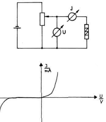
current running through the voltmeter. The current must therefore be corrected. Concerning the circuit diagram on the right ("Spannungsfehlerschaltung") the voltmeter also measures the voltage across the ammeter. This error must also be corrected. To this end, the given internal resistances of the measuring instruments can be used. Another systematic error is produced by the uncontrolled temperature increase of the semiconductor element, whereby the electric conductivity rises.
