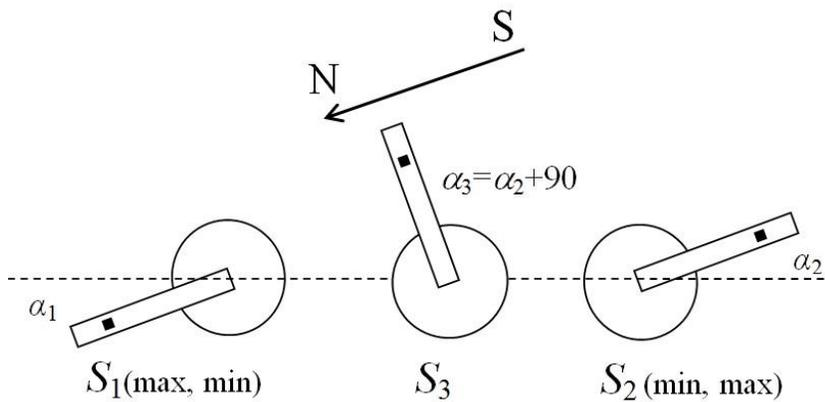
a. Orient the sensor along the Earth's magnetic field. Find the direction with the maximum (or minimum) value of  $S$ . Note this value  $S_1$  and the angle  $\alpha_1$  between the sensor direction and the horizontal.
