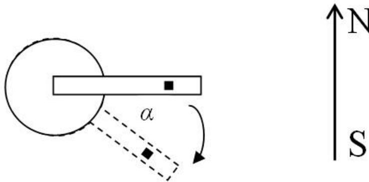
a. Set  $\alpha = 0$  - the sensor perpendicular to the direction South-North.
