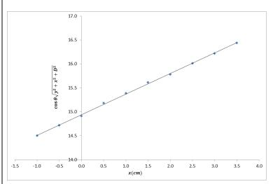
From the plot, we can estimate the slope to get  $\phi^* = 23.2^{\circ}$ . (Remark: one can also find out the y-intercept to be D = 14.9 cm, which is in good agreement with the value assigned in this experiment.)
