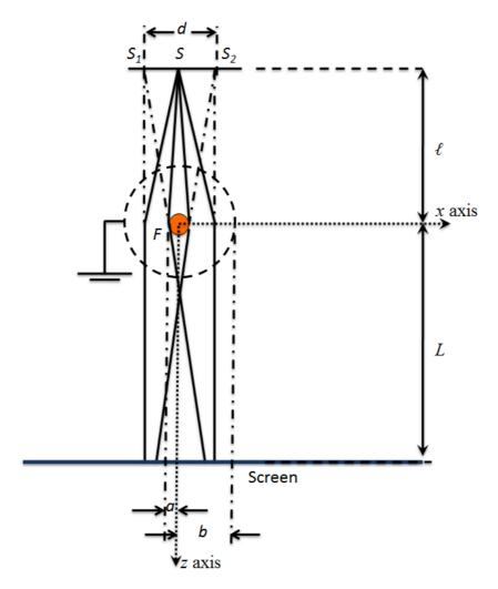
The electron "biprism" consists of a grounded cylindrical wire mesh with a fine filament F at the center. The distance between the source and the "biprism" is  $\ell$ , and the distance between the distance between the "biprism" and the screen is L.
