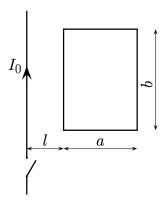
The resistance of the loop is R. The current in the long wire is quickly switched off.
