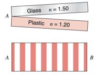
They touch at point A. Light of wavelength  $600 \,\mathrm{nm}$  is incident normally from above. The location of the dark fringes in the reflected light is shown above.
