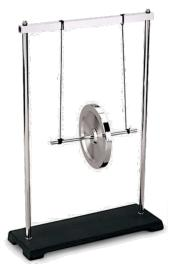
It consists of a uniform disc of mass M and radius R, with a massless axle of radius r. If the wheel is released from rest, it falls downward, in such a way so that the strings supporting it are always perfectly vertical. Find the acceleration.
