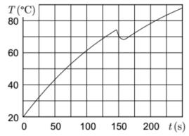
Find the mass of the ice if the heating power of the kettle is  $P = 1 \,\text{kW}$ . The latent heat of melting for ice is  $L = 335 \,\text{kJ/kg}$ , the heat capacity of water is  $c = 4.2 \,\text{kJ/kg}$  K, and the temperature of the room is  $T_1 = 20 \,^{\circ}\text{C}$ . (Hint: it's very easy to get an answer that's off by up to 50% if you're careless.)
