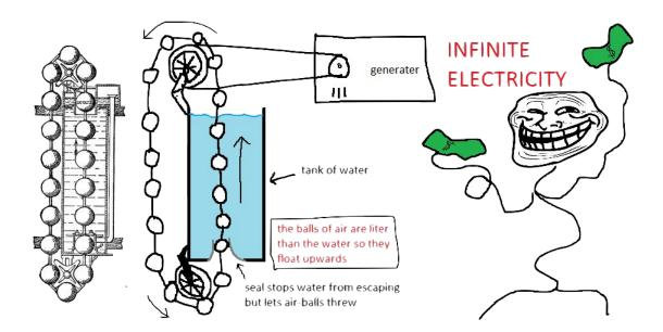
The balls are less dense than water. The balls on the left are pulled downward by gravity, while the balls on the right are pushed upward by the buoyant force. Why doesn't this work? Moreover, can you explain why it still wouldn't work if the balls and chain were replaced with a flexible tube of constant thickness?
