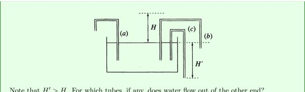
Note that H' > H. For which tubes, if any, does water flow out of the other end?
