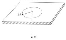
The motion is frictionless. Show that the motion is stable with respect to small changes in the height of m, and find the frequency of small oscillations.
