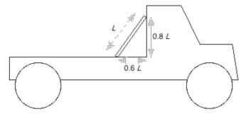
There is no friction between the top of the board and the vertical surface of the truck. The coefficient of static friction between the bottom of the board and the horizontal surface of the truck is  $\mu_s = 0.5$ . The truck always moves in the forward direction.
