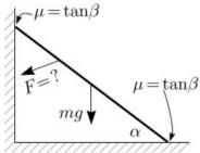
What is the minimum additional force F needed to keep the rod static?
