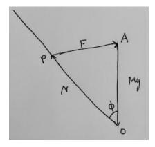
We see that the magnitude of N varies as P varies along the line  $\ell$  which is the line at angle  $\phi$  to AO, and the magnitude of F is AP. AP is minimized when P is the foot of the altitude from A to  $\ell$ , so we see
