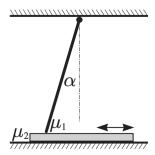
Underneath, a board is being dragged on the floor. The coefficient of (static and kinetic) friction is  $\mu_1$  between the board and rod, and  $\mu_2$  between the board and floor. The rod is meant to stop the board from being dragged to the right, no matter how hard or how quickly it is pulled. Is this possible? If so, what are the conditions on the parameters that allow this to occur?
