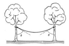
Find the tension at either end of the rope, and the tension at the middle of the rope.
