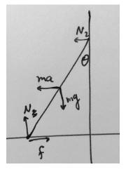
Force balance gives mg = N and  $N_2 + ma = f$ , and torque balance gives
