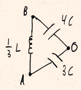
This is now a simple LC circuit with  $L_{\rm eff}=(1/3)L$  and  $C_{\rm eff}=(12/7)C$ , giving the final resonant frequency  $\omega_3=\sqrt{7/4LC}$ .
