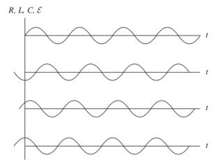
Which is which? Whose impedance is larger, the inductor's or the capacitor's?
