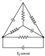
The capacitors have capacitance C, the inductors have inductance L, and the resistors have resistance  $R = \sqrt{L/C}$ . Furthermore, the driving frequency is  $\omega = 1/\sqrt{LC}$ . Find the amplitude of the total current through the circuit.
