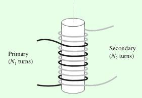
The "primary" coil has  $N_1$  turns and the secondary has  $N_2$ . If the current I in the primary
