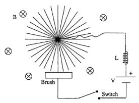
A battery with voltage V feeds current through an inductor L, into the axle, through the spoke, to the brush. There is a uniform magnetic field  $\mathbf{B}$  pointing into the plane of the paper. At time t=0 the switch is closed.
