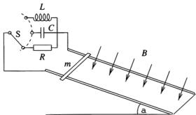
How does the rod move, after being released from rest, if the circuit is closed by (a) a resistor of resistance R, (b) a capacitor of capacitance C, or (c) a coil of inductance L? In all cases, neglect the self-inductance of the closed loop formed, i.e. neglect the flux that its current puts through itself.
