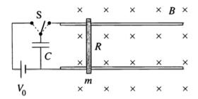
A frictionless conducting rod of mass m, length  $\ell$ , and resistance R is placed perpendicularly onto the track. The capacitor is charged so that the rod is repelled from the capacitor when the switch is turned. This arrangement is known as a railgun. Neglect self-inductance throughout this problem.
