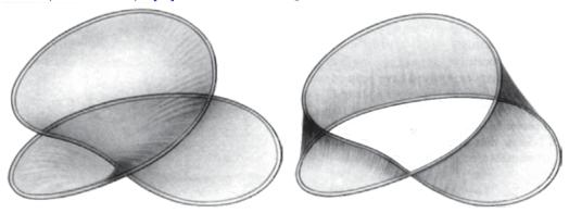
Suppose we want to calculate the flux of  $\mathbf{B}$  through this loop. Two surfaces bounded by the loop are shown above. Which, if either, is the correct surface to use? If each of the two turns in the loop are approximately circles of radius R, then what is the flux? Generalize to an N-turn coil.
