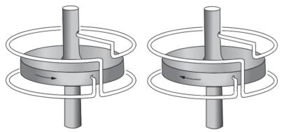
It has only two essential parts. One part is a solid metal disk and axle which can be driven in rotation. The other is a two-turn "coil" which is stationary but is connected by sliding contacts, or "brushes", to the axle and to the rim of the revolving disk.
