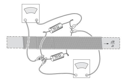
Find the readings on the two voltmeters in terms of  $d\Phi/dt$ , paying attention to the signs.
