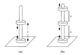
Treat the magnets as dipoles with mass  $m_d$  and dipole moment  $\mathbf{m}$ , with directions as shown above.
