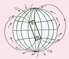
Since the tangential component of this dipole field points north, the red end of the compass points towards the geographic north pole, which is the Earth's magnetic south pole.
