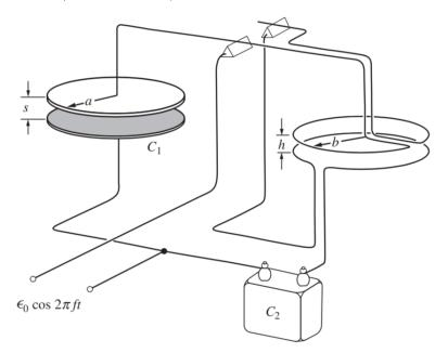
The force between capacitor plates is balanced against the force between parallel wires carrying current in the same direction. A voltage alternating sinusoidally with angular frequency  $\omega$  is applied to the parallel-plate capacitor  $C_1$  and also to the capacitor  $C_2$ , and the current is equal to the current through the rings. Assume that  $s \ll a$  and  $h \ll b$ .
