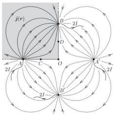
Here, the plate is now infinite, and we have a new current source and sink respectively at the reflections of A and B in O. Now, if a current 2I enters the plate, the current at a distance r is  $\frac{2I}{2\pi rt}$ , so the electric field at a distance r is  $\frac{\rho I}{\pi rt}$  (pointing radially outward), so the potential is  $\frac{\rho I}{\pi t} \log(r/r_0)$  for some arbitrary  $r_0$ . For our purposes, set the potential to be 0 at O, so  $r_0 = AO$ . Now,
