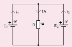
For example, in the above circuit, Kirchoff's rules don't determine the currents; they only say that  $i_1 + i_2 = 1$  A. If the emfs of the batteries were different, the situation would be even worse: the equations would be contradictory, with no solution at all! In real life, this is avoided because all batteries have some internal resistance. Adding such a resistance to each battery, no matter how small, resolves the problem and gives a unique solution.
