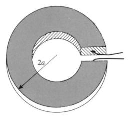
Find the resistance of the washer. (Hint: first argue that no current flows radially.)
