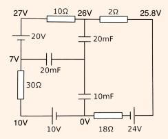
To finish the problem, we need to know the voltage  $V_0$  of the central node, so we need one more equation. That equation is charge conservation: the fact that the central part of the circuit, containing the inner plates of the three capacitors, begins and remains uncharged. Suppressing units, this means
