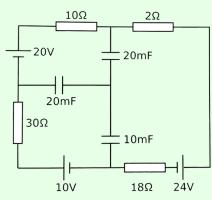
After a long time, what is the charge stored on the 10 mF capacitor?
