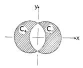
The current in each conductor is uniformly distributed. Find the magnetic field in the space between the conductors.
