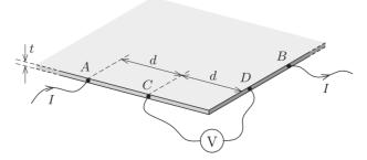
Points A and B are both 2d from the corner, whereas C and D are each a distance d from it. The length of the plate's sides is much greater than d, which, in turn, is much greater than the thickness t of the plate. If a current I enters the plate at point A, and leaves it at B, then the reading on a voltmeter connected between C and D is V. Find the resistivity  $\rho$  of the plate material.
