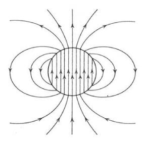
This is an example of a magnetic dipole field. Note that it looks very similar to an electric dipole field far away, but inside the dipole the field points along the dipole moment, rather than against it. This is necessary to make the magnetic field lines form closed loops, and hence obey Gauss's law for magnetism.
