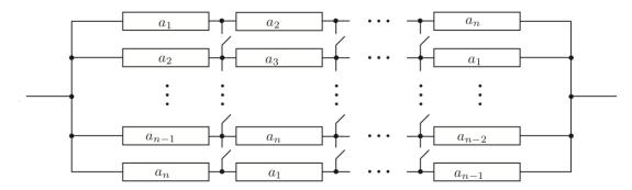
By closing all the switches, show that the arithmetic mean of n numbers is at least the harmonic mean.
