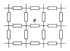
Find the equivalent resistance between two neighboring points by considering the superposition of 1 A flowing into one point, and 1 A flowing out the other.
