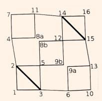
This is valid because the separated nodes 8a/8b and 9a/9b still have the same potential in the new network, by the diagonal symmetry. (This is using the above idea in reverse.) Now, the circuit has been reduced to combinations of series and parallel resistors. The resistance between 1 and 2/3 is R/2. The resistance between 2/3 and 14/15 is the combination of three networks in parallel, and finally the resistance of 14/15 and 16 is R/2. Thus,
