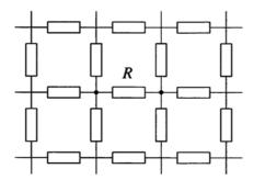
Find the equivalent resistance between two neighboring points by considering the superposition of 1 A flowing into one point, and 1 A flowing out the other.
