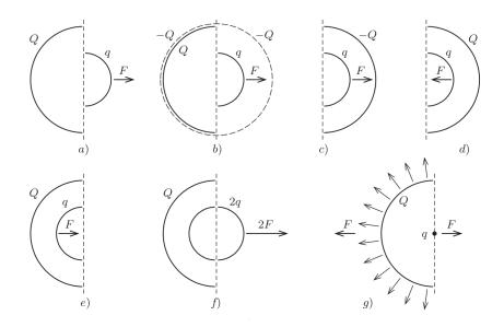
The force we want to compute is shown in (a). Now consider superposing a uniformly negatively charged sphere with radius just larger than R, as shown in (b). By the shell theorem, this doesn't change the force on the hemisphere of radius r. The result of the superposition is (c). Flipping the charge of one of the hemispheres in (c) flips the force, leading to (d). Finally, reflecting (d) gives (e).
