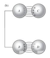
The spheres C and D induce charges of opposite sign on A and B. Now suppose C and D are connected by a wire. Then the charge distribution should not change, because the charges on C and D are being held in place by the attraction of the opposite charge density. Is this correct?
