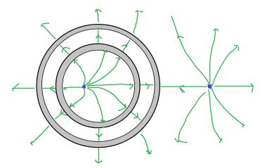
Whether or not there are any field lines coming from the charge outside the shell depends on how close that charge is to the shell. (The entire field configuration in this problem can be found exactly using the method of images, as shown in **E2**.) In the case that the two spheres are connected with a wire, the field in between the two spheres disappears, but nothing else changes.
