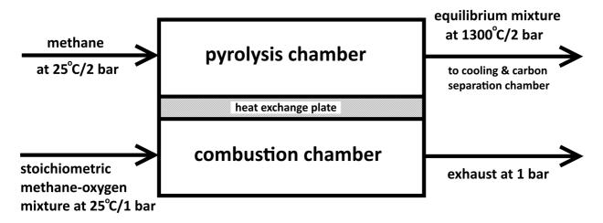
2. Calculate the total quantities (in moles) of methane and oxygen required to produce one mole of hydrogen using the results from question 1 and assuming that a) thermal equilibrium is established between the combustion chamber and the pyrolysis chamber, b) no heat is
