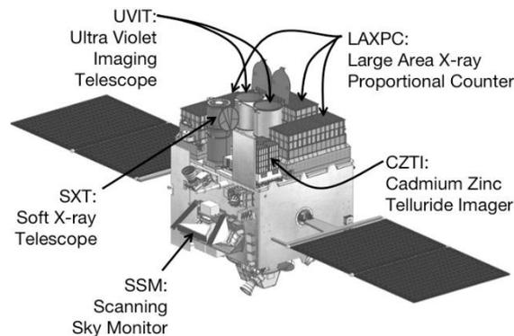
In this question, we will discuss three of these instruments (SXT, LAXPC, CZTI), which point in the same direction and observe in X-ray wavelengths. The details of these instruments are given in the table below.
